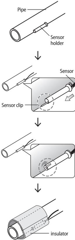
When the pipe is not a copper pipe
