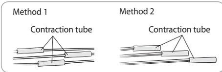
6. Wrap it with the insulation tape twice or more and position your contraction tube in the middle of the insulation tape.
