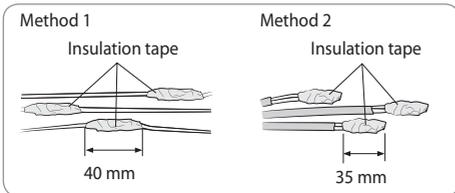
7. After tube contraction work is completed, wrap it with the insulation tape to finish.
