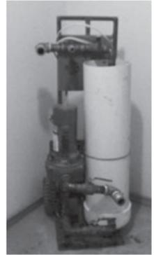
Flushing unit (or purging cart)
