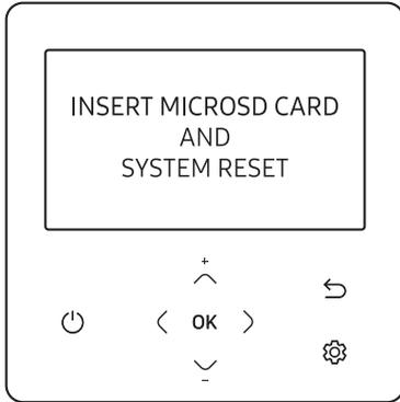
1. When you remove the microSD Card during download, the “INSERT MICROSD CARD AND SYSTEM RESET” screen appears and the download is stopped.
