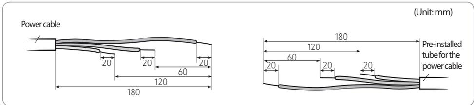
3. Insert both sides of core wire of the power cable into the connection sleeve.
